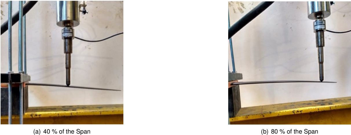
Figure 4.1: Experimental set for point loading analysis at 40 % span (left) and 80 % span (right) [6]
